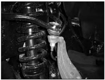
10. Support the lower control arm with an appropriate jack. Remove the three upper strut mounting nuts at the frame. (Fig 6) DO NOT remove the center strut rod nut. Save nuts.
