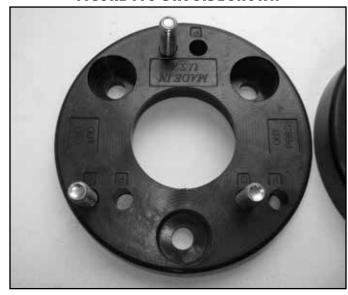
17. 2009-2013 model years: Install the new spacer on the strut and fasten with the original mount nuts. The spacers are labeled to indicate which side will face 'out' on the vehicle once they are installed. The studs need to be opposite of the factory studs and the assembly will only fit on the strut one way. (Fig 12)
