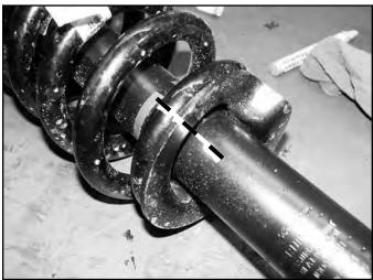
**Caution** Coil Spring is under extreme pressure. Improper removal/installation of coil spring could result in serious injury or death. Use only a high-quality spring compressor and carefully read and follow the manufacturer's instructions.
