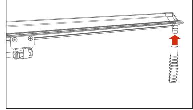
Place the passenger side rail (A) on to the passenger side mounting rail (N) installed in the previous steps. Position the side rail flush with the top edge of the mounting rail. The end of the side rail with the drain tube goes toward the cab of the truck.
