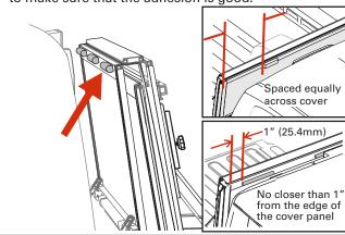
Unfold the cover toward the tailgate. Then confirm each panel is centered side to side and front to back on the truck bed. If adjustments are needed, loosen the cover retainer clamps (E) and shift the cover until it is positioned correctly. The rear edge of the cover and tailgate seal should rest on top of the tailgate. For proper sealing, the tail panel will overlap by .5".
