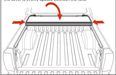
Confirm the retainer clamps (E) are positioned around the side rails (A & B) correctly as shown below. Tighten the retainer clamps by turning them clockwise until the lock washer is secure.
