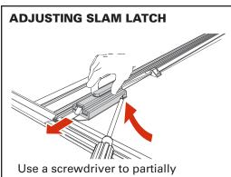
Use a screwdriver to partially pry open the tab on the latch housing. At the same time slide the housing away from the latch assembly.
