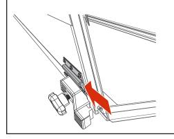
First, prep the buckle ends (G) by peeling off the adhesive liner of the gasket (J).
