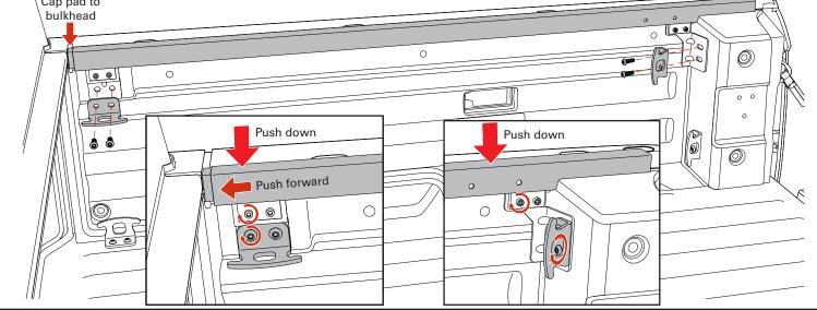
Insert the passenger rail end corner (V) into the tailgate end of the passenger side mounting rail (N).
