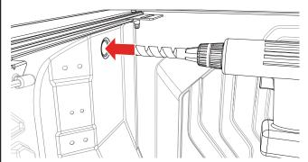
Insert the drain hose (J) into the drilled hole in the bed. Slide the collared end of the hose onto the cover rail drain. Install the other half of the hose on the passenger side in the same manner.
