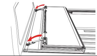
**FLIPPED UP POSITION:** Fold the cover (A) open and lift it until it's vertical or past 90 degrees towards the truck cab. Then release the prop rod that is attached to the rail. Fold the prop rod over and position it firmly against the vertical plate on the underside of the cover. Then slide the prop rod locks downwards and tighten the
