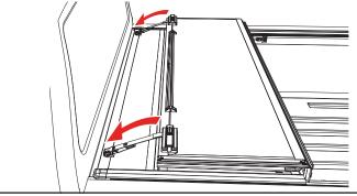
**FLIPPED UP POSITION:** Fold the cover (A) open and lift it until it's vertical or past 90 degrees towards the truck cab. Then release the prop rod that is attached to the rail. Fold the prop rod over and position it firmly against the vertical plate on the underside of the cover. Then slide the prop rod locks downwards and tighten the
