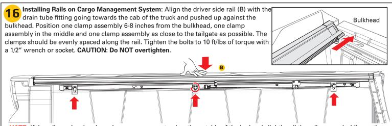
**NOTE**: If the rails are leaning down, have one person stand on the outside of the bed and slightly roll the rails upward while another person slowly snugs the clamps up. If the clamps are tightened too quickly or overtightened, it will cause the rails to lean down.
