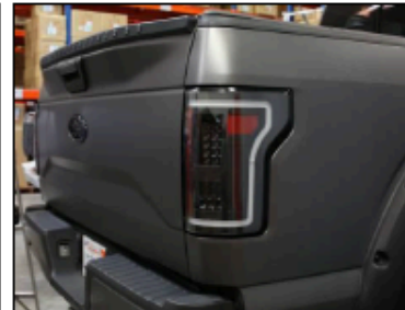
Repeat steps 2-8 for other tail light. Test all functions of lights before driving vehicle.
