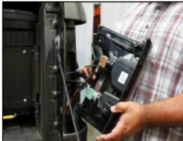
Connect both factory connections and resistor to Anzo USA tail light.
