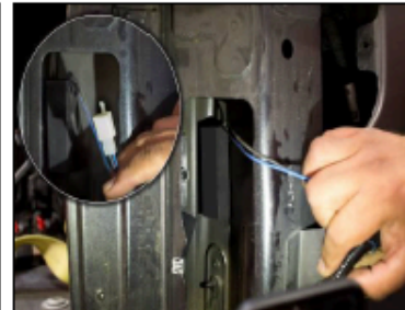
Peel 3m tape backing from resistor and press resistor securely in fender well.
