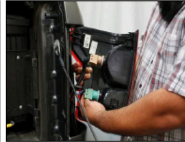
Hold tail light secure in hand and pull tail light towards back of vehicle to remove.
