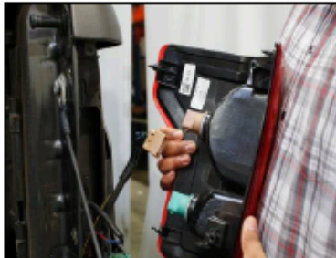
Disconnect both connections from factory tail light.
