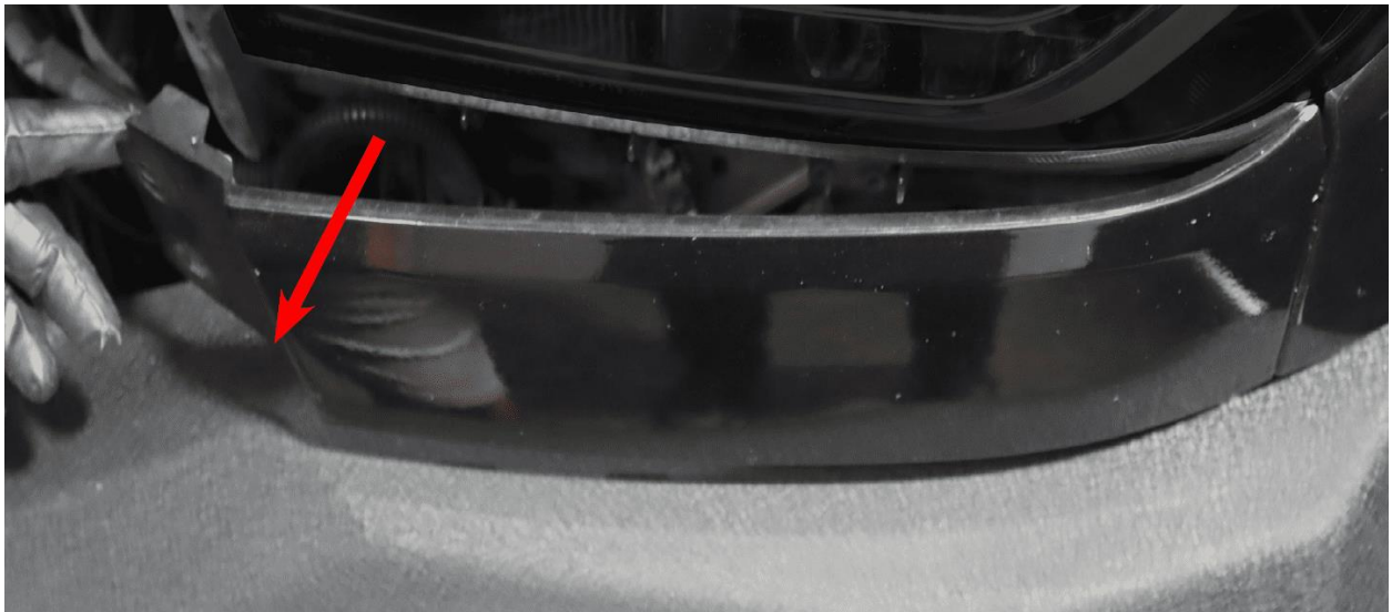
Use the plastic panel popper to help you release the side joint pins.
