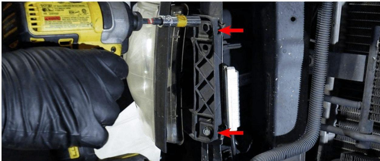
Take out the 2 plastic retainers by utilizing a screwdriver.
