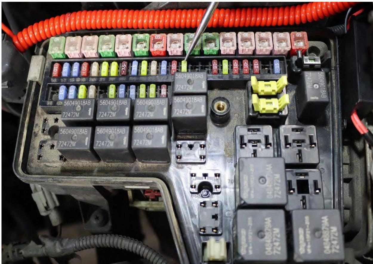
Crimp the gray wire from the harness to the fuse tap and connect it to fuse #29 (20A). After completing this step, route the wire and close the fuse box cover.
