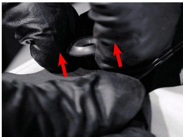
Utilize an extension to remove the 10mm bolt located at the bottom of the headlight. Repeat the same steps to remove the headlight on the other side.
