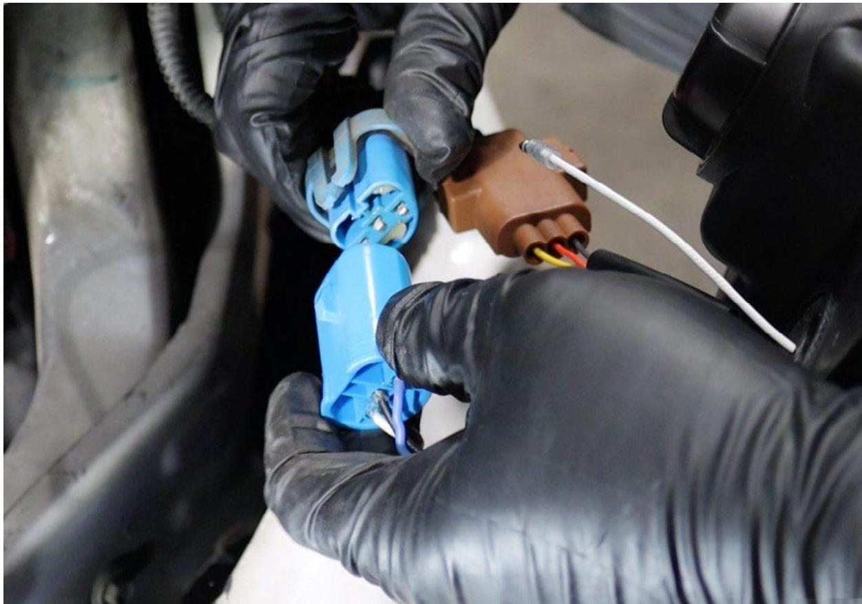
Secure the harness to the daytime running light connection on the back of the headlight.
