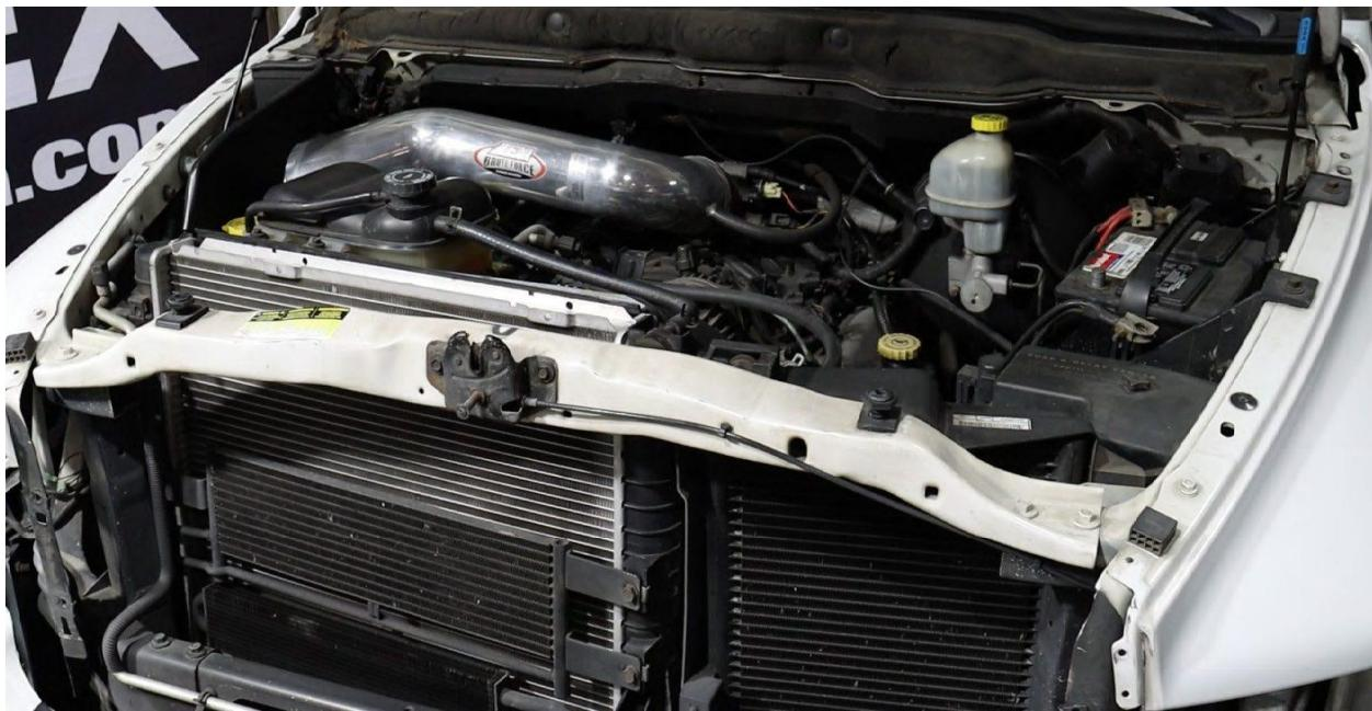
Connect the red wire to the battery's positive terminal and the black wire to the battery's negative terminal or the 10mm bolts on the firewall.
