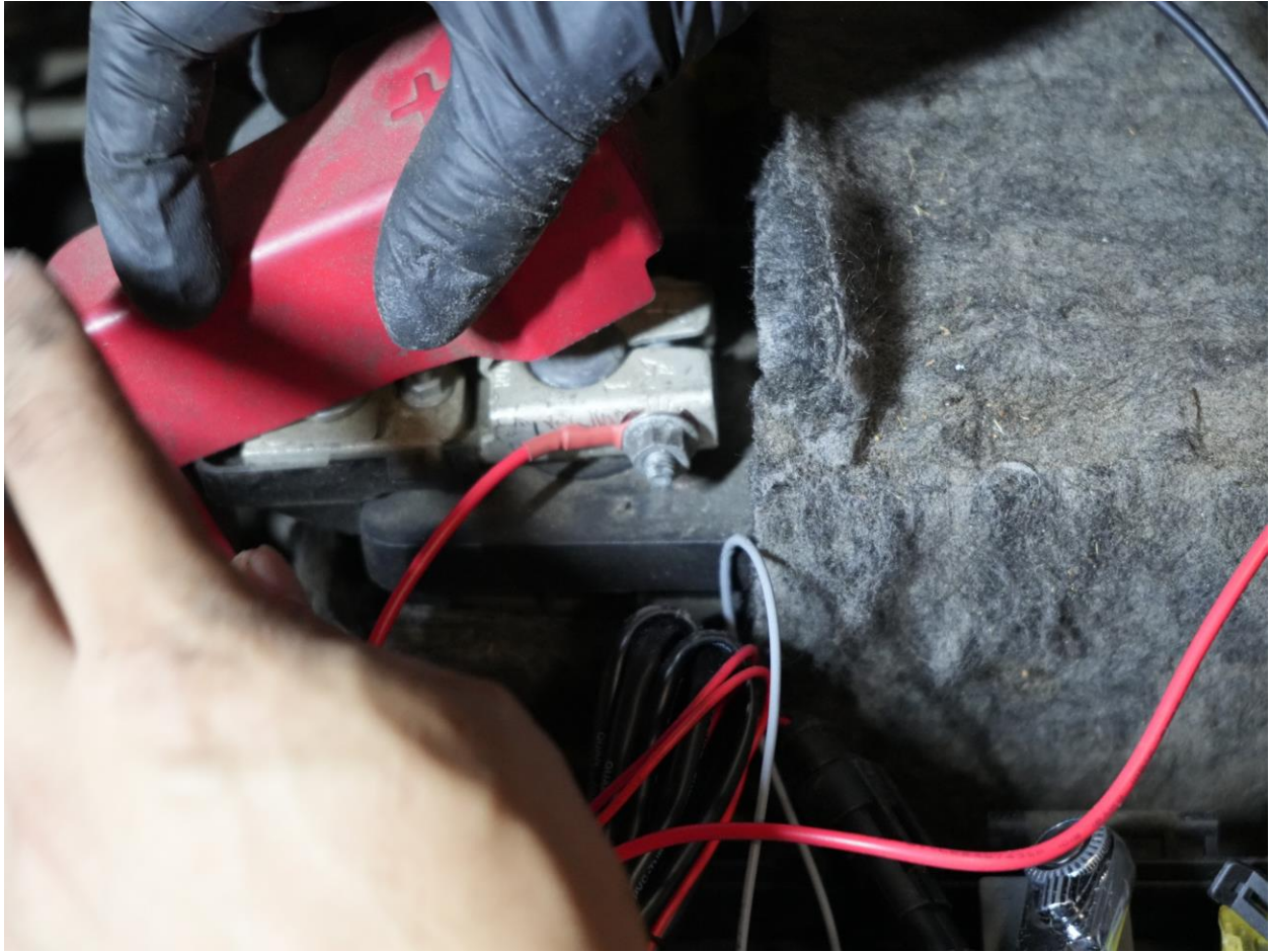
Route the daytime running harness to the location of both
