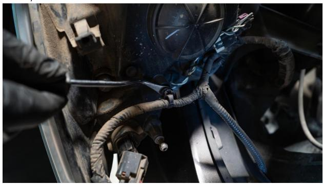
Keep in mind that the larger plug is for the turn signals, while the smaller plug is for the low and high
