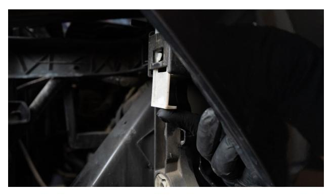
With the locking clip released, you can now carefully pull the headlight assembly away from the vehicle.
