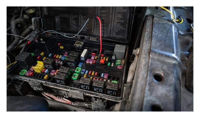
Now move on to the bullet connectors on the red wires:
