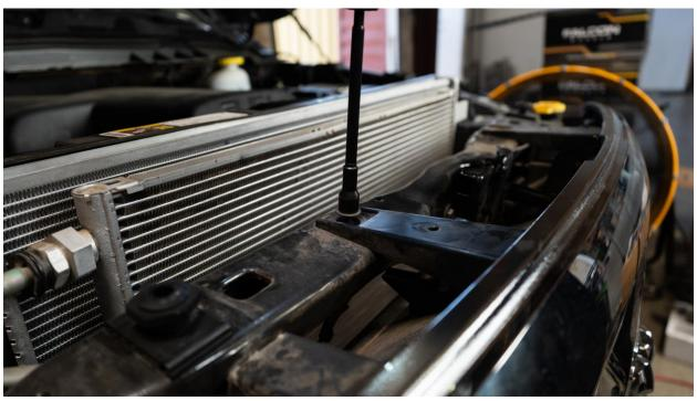
With all four bolts removed, firmly pull on the lower portion of the grille to release it—it may require a bit of force to pop it free.
