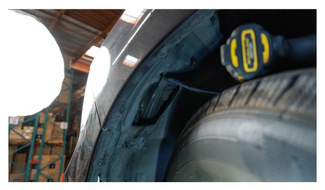
With the hatch opened, reach inside and locate the locking clip. To release the headlight, pull the clip back and then push it upward until it disengages.
