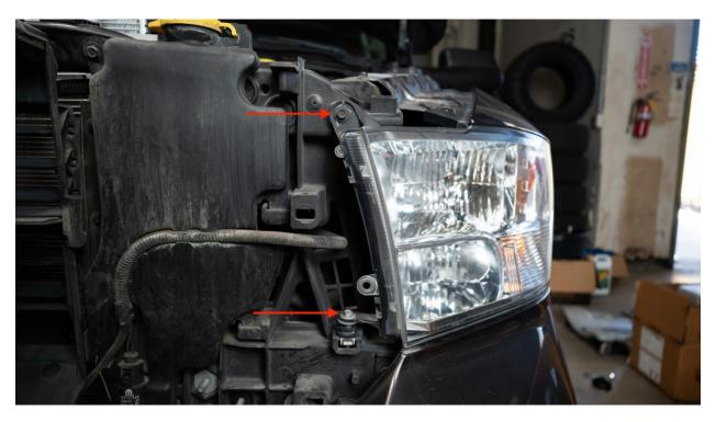
After removing the two bolts, you can move on to releasing the locking clip at the back of the headlight. To access it, open the "hatch" in the wheel well liner—this panel is held in place by a single clip that will need to be removed.
