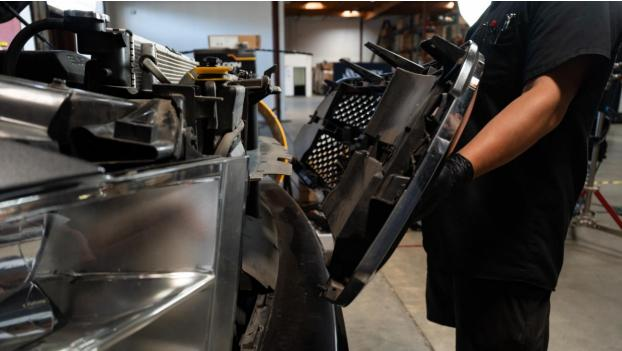
With the grille removed, you now have access to the headlight. It is secured by two 10mm bolts at the front and a locking clip at the back that will need to be released.
