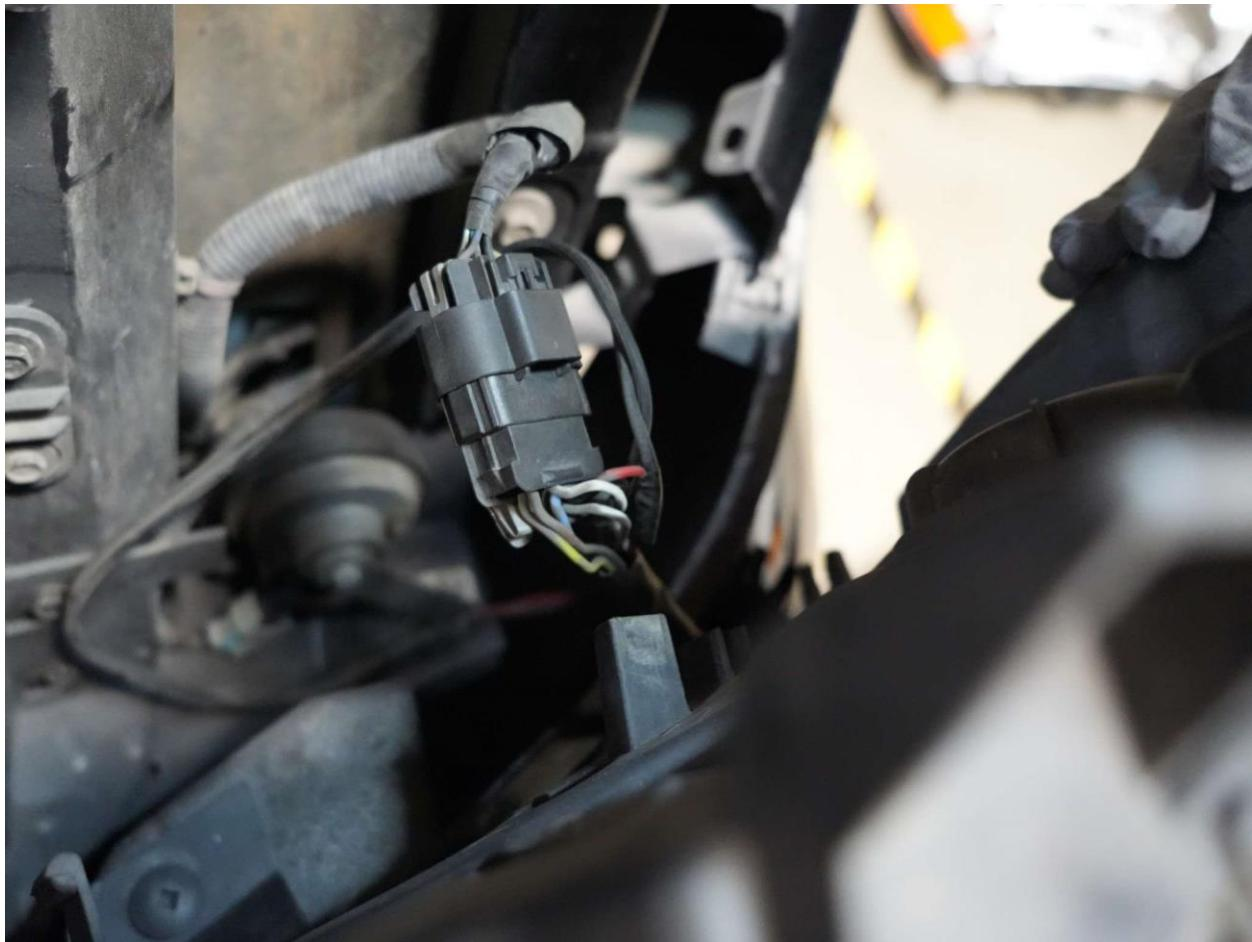
Install the headlight onto the vehicle by reversing the steps from the removal process. Ensure it is secured with the two 10mm bolts.
