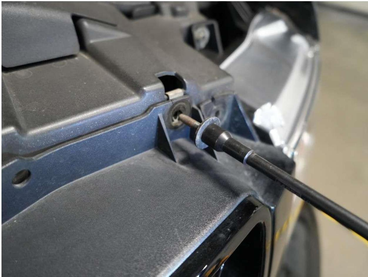
Next, remove the two 7mm bolts and the two push-in pins from the front wheel well. Then, open the inner liner to reach inside for the three 10mm bolts securing the side of the front bumper
