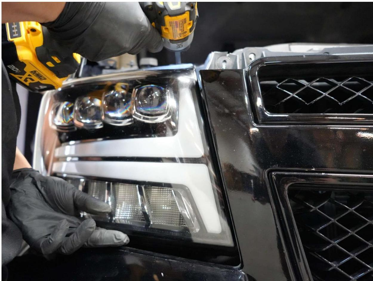
Complete the headlight installation by reversing the removal process. Carefully reinstall the front bumper by securing all the bolts to ensure it is properly mounted.
