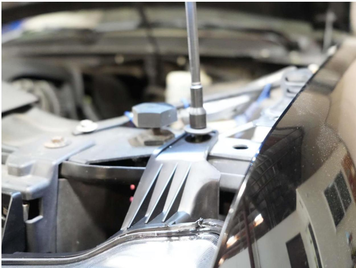
Remove the headlight assembly by gently pulling it outward at a slight angle from the side, then continue pulling it straight towards you. Disconnect the headlight socket to fully remove the assembly. Repeat this step for the other side.
