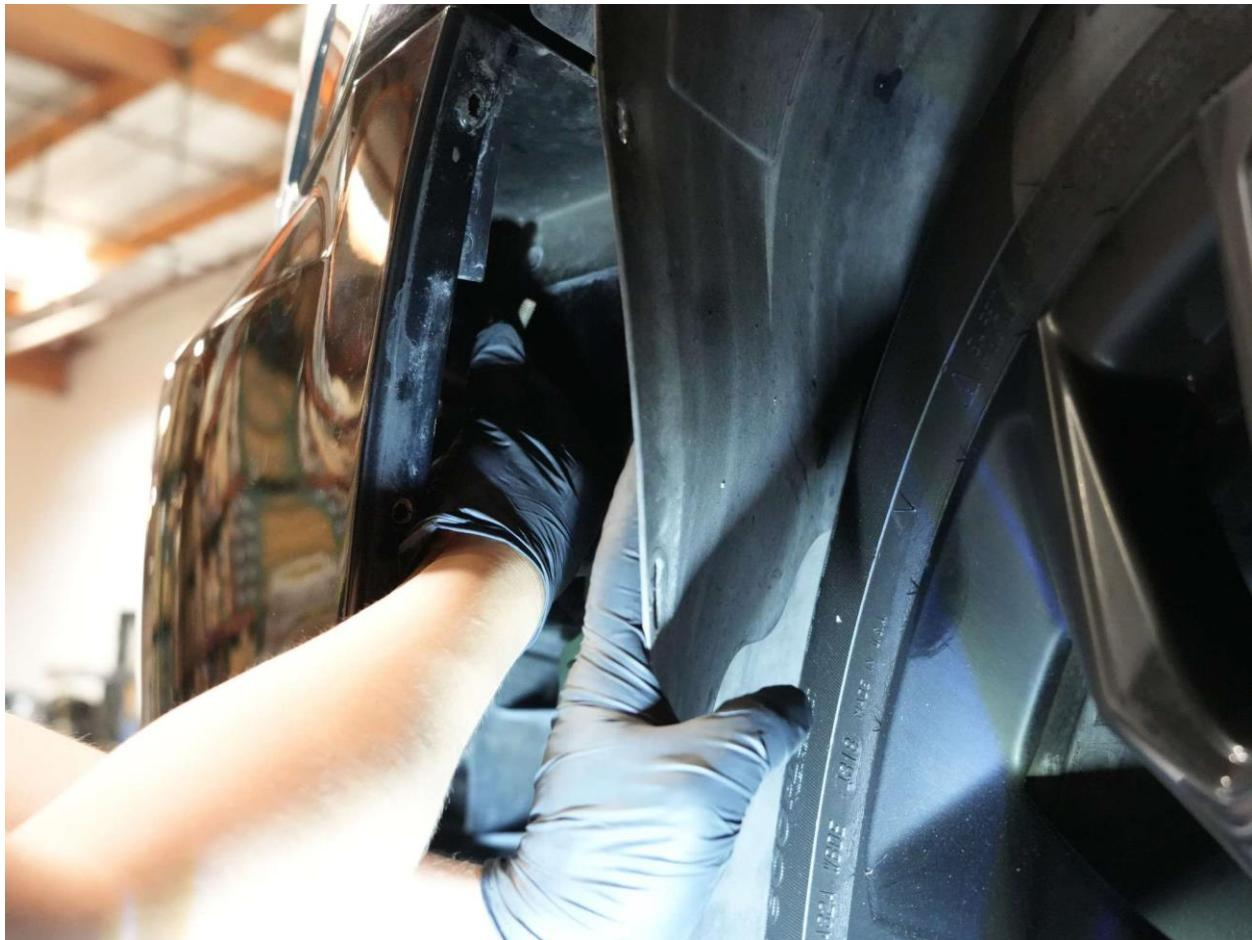
When reaching inside the inner liner, you will see the three 10mm bolts securing the front bumper. Remove these bolts.
