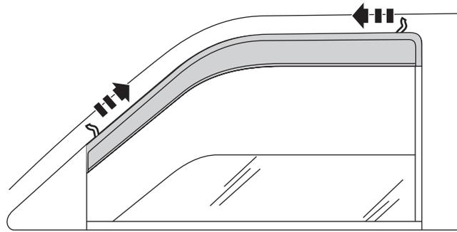
Apply pressure along all flanges to ensure proper adhesion of tape.
