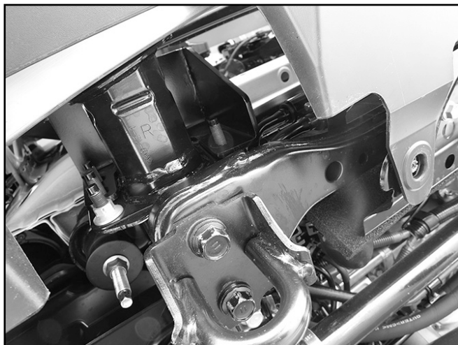
(Fig 5) Passenger side Top Bracket pictured installed over bumper bracket. Pictured from below. On 14-17 models, insert Top Bracket up from below bumper and rotate into position over bumper bracket mounting studs.
