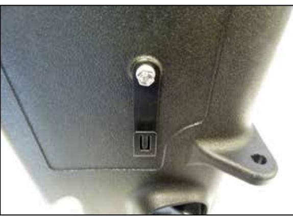
11. Install the provided wiring harness bracket onto the AIRAID® air filter housing and secure with the provided hardware.
