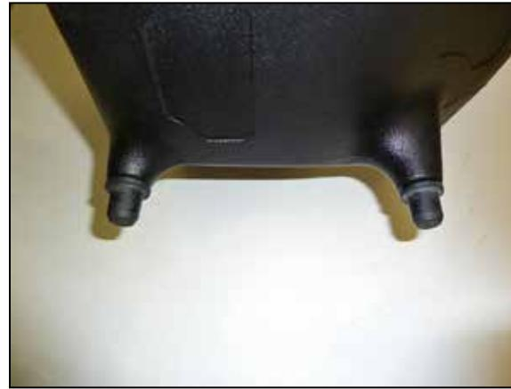
12. Remove the two factory mounting grommets from the factory air filter housing and install them onto the AIRAID® air filter housing.
