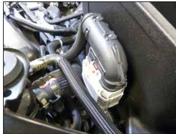
15. Clip the wiring harness onto the bracket installed onto the AIRAID® air filter housing.
