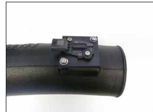
19. Install the mass air sensor assembly into the AIRAID® intake tube in the direction shown and secure with the provided hardware.
