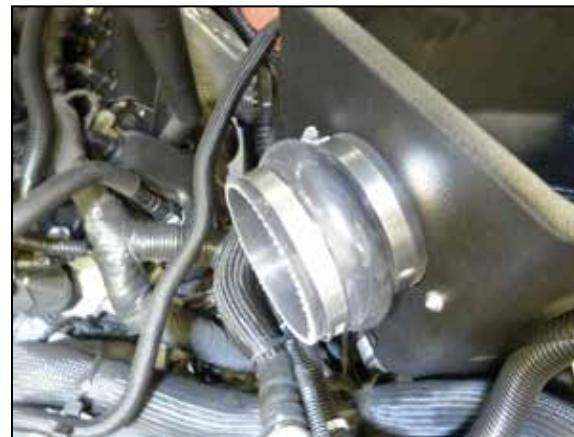
16. Install the provided hump coupler onto the filter adapter and secure with the provided hose clamp.
