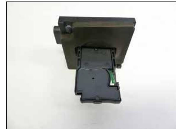
18. Install the provided gasket onto the provided mass air sensor adapter. Remove the mass air sensor from the factory air filter housing and then install it into the adapter and secure with the provided hardware.
