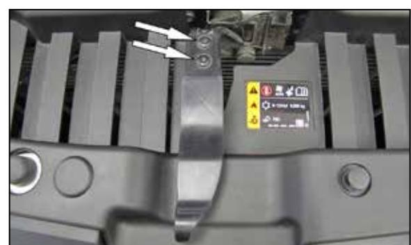
5. Remove the two bolts that secure the hood release arm to the hood latch and then remove the release arm.
