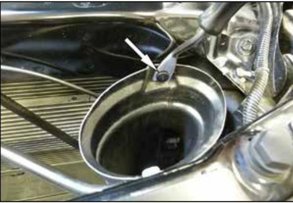
7. Remove the plastic clip securing the fresh air intake duct onto the core support, then pull the duct forward to disengage it from the factory air filter housing.
