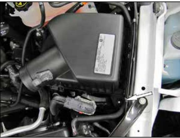
9. Remove the nut that secures the air filter housing assembly to the vehicle. Remove the air filter housing assembly from the vehicle.
