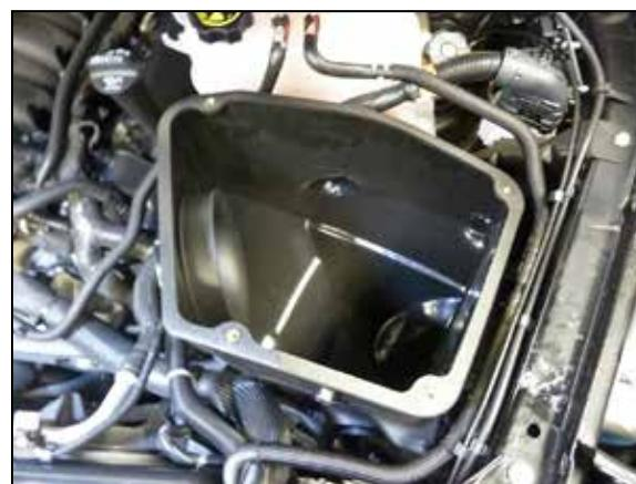
13. Install the AIRAID® air filter housing into the vehicle so the mounting grommets engage into the factory mounting holes. Secure the housing with the factory nut removed in step #9.
