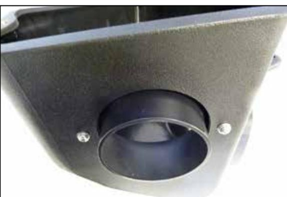
10. Install the provided radius filter adapter into the AIRAID® air filter housing and secure with the provided hardware.
