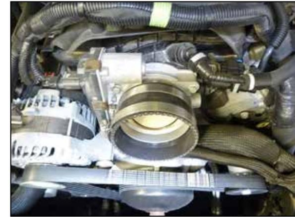
17. Install the appropriate coupler onto the throttle body. The 5.3L engine will use the smaller coupler and the 6.2L engine will use the larger coupler. Secure with the provided hose clamps.
