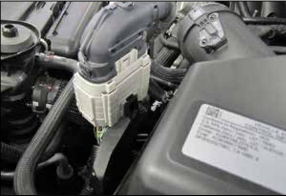
8. Using a small 90° pick or similar tool, release the locking tap that secures the wiring harness bulk connector to the air filter housing and then unhook the connector from the housing. Unhook the wiring harness from the two locations held with tie wraps.
