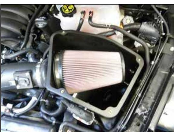
24. Install the AIRAID® air filter onto the filter adapter and secure with the provided hose clamp.
