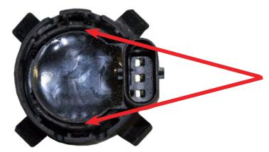
Spread these tabs and release the parking sensor from the rear
