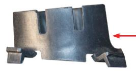
Install this backing ring with the slimmer part faced towards the center of the bumper.
