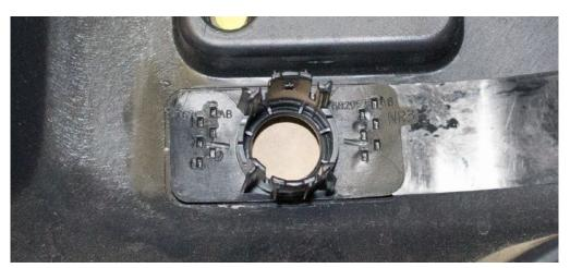
Use a scraper to separate the mounting plate from the bumper
