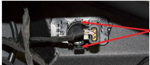
Spread these tabs to release the sensor
