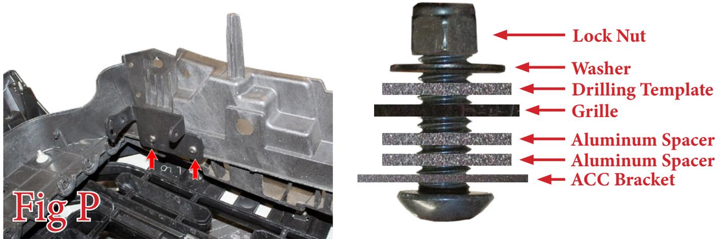
18. Set the rest of the bracket and module in place. Use the supplied Black 1/4" Bolts (x4), Black 1/4" Washers (x4) and Black 1/4" Lock Nuts (x4) as well as the supplied 1/4" Carriage Bolt (x1), 1/4" Washer (x1) and 1/4" Lock Nut (x1). (Fig Q) **Make sure to adjust the tilt on your Adaptive Cruise Module so that the module is parallel to the front face of the grille, and perpendicular to the ground.**
