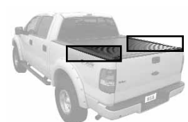
End slat lining up with tailgate & side rail. (1/16" gap between end slat and side rails)
