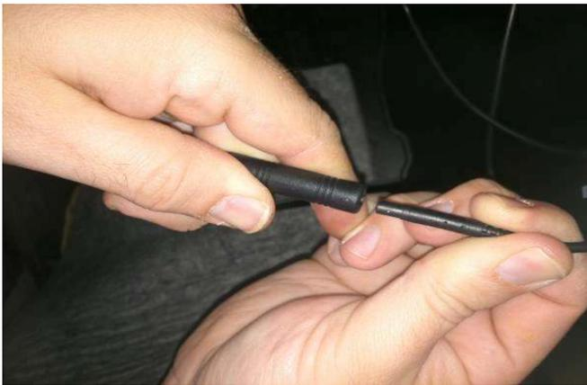
**Step 10: Plug the new connector into the factory connector that the factory camera was just unplugged from.** Make sure that the new connector "clicks" into place.
