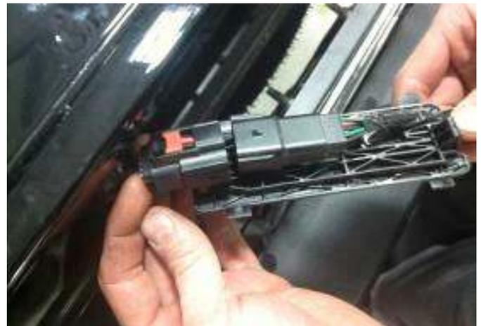
**Step 8: Run the new camera harness through the opening in the back of the bed to the underside of the vehicle.**
