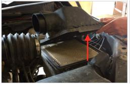
7. Remove the retaining bolt on the stock air box using a 13mm socket. Note: The retaining bolt will be reused again in Step 18.
