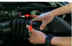
3. Unlatch the two latches on the stock air box.
