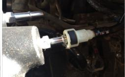
**25.** Reconnect the PCV hose. Push in the connector over the Quick Connect Fitting (Q) until you hear it snap into place.
