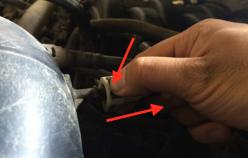
8. Remove the plastic rivets on the stock air scoop using a flat head screwdriver.
