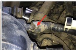
9. Lift and remove the stock air box.
