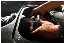
22. Tighten the Hose Clamp #88 (J) at the Air Filter (D).
