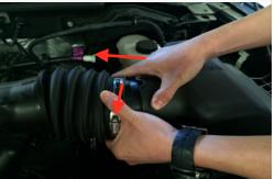
4. Lift and remove both the lid and air filter.
