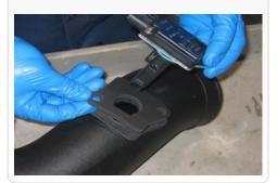
gauge is inserted completely into the grommet of the intake tube.
