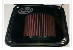
28. For increased airflow we recommend using the provided Inlet Lid, to seal off the box completely from foreign objects use the provided Clear Lid.
