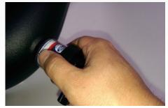
18. Slip the Hump Adapter (N) along with two #72 hose clamps (V) over the Intake Tube (C) until nearly flush with the end.
