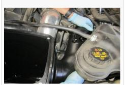
20. Place the Intake Tube (C) through the tube seal of the air box.
