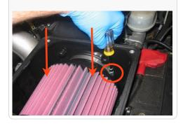
25. Reconnect the restriction gauge to the harness. **NOTE:** <u>DO NOT</u> rely on the OE restriction gauge or wait until the dash light is triggered before you service your S&B air
