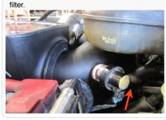
**26.** Reconnect the electrical connector to either the MAF sensor or Temp. Sensor located on top.
