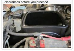
11. Spread the OE clamp open and remove the breather tube assembly from the OE intake tube.
