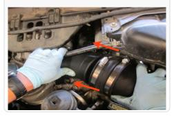
23. Secure both #72 Hose clamps after both tubes and coupler are aligned together
