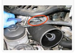
Temp. Sensor NOTE: If your vehicle uses a Temp. Sensor in place of a MAF Sensor: Use the supplied Temp. Sensor grommet (M) and install it in the hole of the intake tube (C). Once the grommet is installed insert the Temp Sensor into the grommet.
