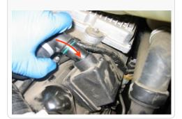
15. Use the supplied T-20 Torx tool and remove the MAF sensor from the OE intake.
