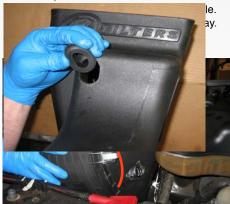
/. Prior to installing the Air Box (A), you may need to rotate the factory intercooler clamp that is located just below the OE air box to add clearance for the new one
