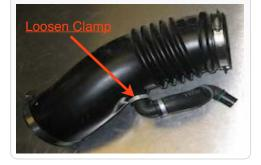
**14.** Insert the OE breather tube assembly into the valve cover.
