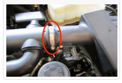
5. Undo the three clips holding the air box cover to the air box. Remove the air box lid and air filter from the truck.
