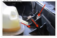
Remove the other air box mounting bolt using 13mm socket. Carefully tip the air box assembly away from the fender so that coolant isn't spilt.
