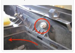
8. Pull the assembly out of the factory grommets and remove from truck. Note: You will have to remove the bolt from the rubber tube to fit through the air box assembly.
