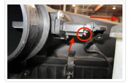
4. Loosen the hose clamp at the air box/ intake tube connection. Then remove the intake tube assembly from the truck.
