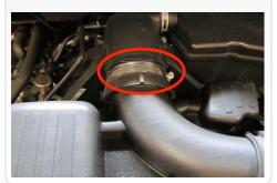
3. Disconnect the MAF sensor by sliding the red locking pin back, press in the bottom of the harness and pull out the male connection.
