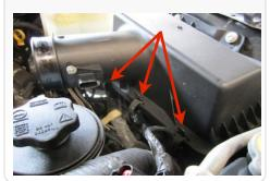
6. Using a 13mm socket, remove the rear air box mounting bolt. Then carefully remove the coolant overflow tube from the reservoir and use the mounting bolt as a temporary plug for the tube.
