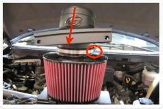
20. Slide the Filter assembly into the Air Box. Install two #80 Hose Clamps (H) over the Hump Adapter (Q). Push the Hump hose over the end of the Adapter Tube (F).
