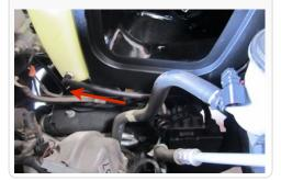
17. Remove the coolant from the OE reservoir and pour it into the Coolant Recovery Tank (B). Note: It may be necessary to add coolant to meet fill range of the new tank. Be sure to use Foot
