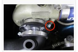
14. Hook the latch on the Intake Tube (L) to the bottom edge of the Air Box (P). Secure the tube to the box using the 2 supplied 5/16 SS Screw (M).
