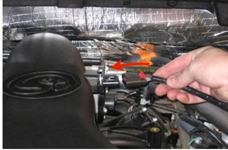
23. Install the Crank Case Vent Hose (A) at the valve cover and Intake Tube (C) on the Passenger's side. Secure both ends using the #8 Hose Clamp (B).
