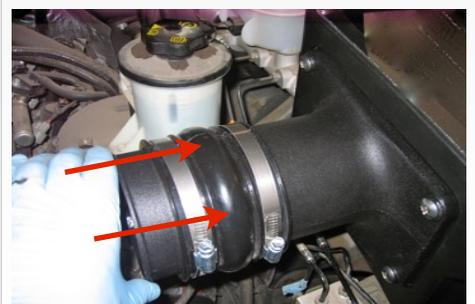
18. Install the Step Adapter (E) over the Intake Tube (C) and secure using a #60 Hose Clamp (D). **Note:** You may find it easier to install the Adapter (E) on the throttle body first then install the Intake Tube (C) in Step #21.
