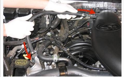
24. **IF EQUIPPED:** Attach the OE brake boost vacuum line to the Intake Tube (C) on the Driver's side and secure using a #8 Hose Clamp (B). Caution: Intake Tube (C) must be modified if equipped with vacuum line. See step #4
