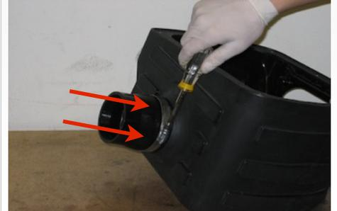
13. Place the Rubber Spacer (L) over the holes on the fender.
