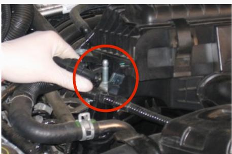
8. Pull up at the throttle body to remove the intake assembly from the vehicle.
