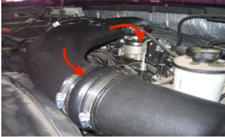
22. Reconnect the MAF sensor electrical connection.
