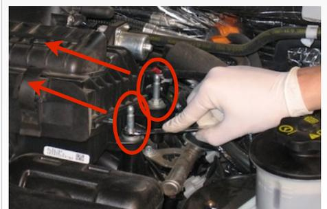
7. Unclip the wire loom from the OE air box.
