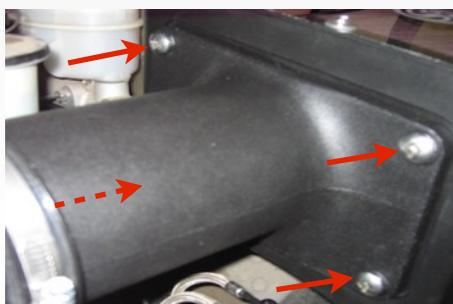
17. Place the Hump Adapter (H) and #72 Hose Clamp (G) over the Filter Adapter (J). Do not tighten at this time.
