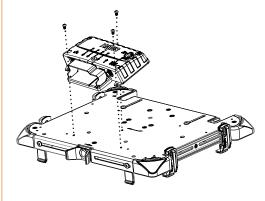
4) Connect all required cables between peripheral devices and Rugged Hub, then reinstall the Strain Relief Bracket as shown with fastener retained from Step 1.
