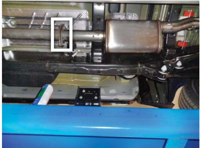
10. Adjust the exhaust components to provide a satisfactory fit. Maintain a minimum of 1/2" clearance around all components of the exhaust system, keeping in mind suspension, travel and vibration. After making any required adjustments, securely tighten the clamps.
