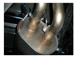
2) Loosen the two clamps at the back of the muffler and carefully slide the tailpipes toward the rear to remove from the muffler. Allow the pipes to hang until installation of the Flowmaster muffler.
