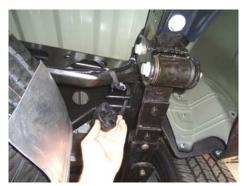
5) Remove the 3 factory rubber exhaust isolators from the mounts on the vehicle, two just forward of the rear axle and one at the rear of the vehicle.
