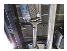
2) Connect the flange on inlet pipe assembly **#26713M** to the factory flange behind the flex pipe, and support the rear of the pipe with a stand. Reinstall the two nuts and tighten enough to hold, but still allow for adjustment.
