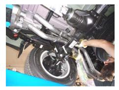
7) Place tailpipe assembly **#86486M** into position over the rear axle and slide into the muffler outlets. Support the rear of the assembly with a stand and connect the rubber hangers on the assembly to the wire mounts on the vehicle. Be sure that the pipes are slid into the muffler about 2.00" and tighten the clamps enough to hold in position.
