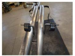
6) Place the rubber isolators removed in the previous step onto the 3 wire hangers of tailpipe assembly **86486M**.
