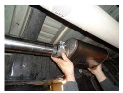
4) Place the provided 3" clamp over the inlet of the muffler, then slide the inlet onto the back of the inlet pipe about 2". Use a stand to support the muffler. Tighten the clamp just enough to hold in position. Place a provided 2 ½" clamp onto each muffler outlet.
