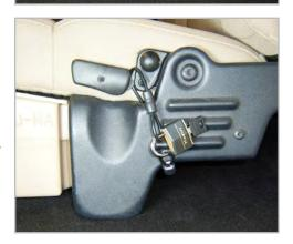
Note: To store lock kit when not in use, remove cable from seat lever and lock around seat bracket only, as pictured below. The lock kit may also be stored inside your DU-HA when not in use.
