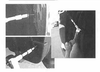
STEP 7: Remove (X6) of the 7mm bolt and retain for installation of Fender Flares.
