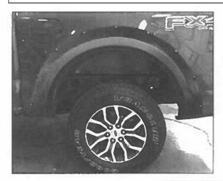
**STEP 13:** Place the Fender Flare onto the vehicle and fit into the correct position following the contours of the body. Using 7.0mm head screwdriver reinstall the previously removed factory spat screws at the upper and lower (A) screw locations through the slots in the front of the Fender Flare at the two noted locations. Re-install the factory retainer clips (B) through the holes in the fender flare at the two noted locations.
