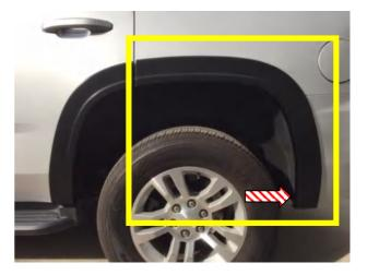
**STEP 11:** Begin installation with rear quarter panel part first. Remove (2) "U" retention clips, (1) Slide-on retention clip, Mylar tape, machine threaded screw and fiber washer from provided hardware. Place Fender Flare onto vehicle in position of best fit. Note rearmost slot in the fender flare.
