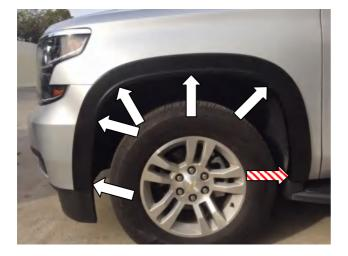
**STEP 7:** Re-install Fender Flare on vehicle in position of best fit. Loosely reinstall the remaining removed #15 torx screw in its previous location at the lowest rear area of the fender. Using the coarse screws and washers, loosely install the (5) remaining attachment points into the nut inserts in the previously installed clips. Ensure part is still in the position of best fit and extrusion is in correct position before hand tightening all screws.
