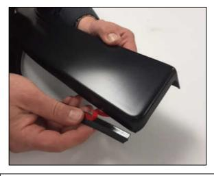
**STEP 8:** Attach the included DOUBLE TAPED rubber seal to the Fender Flares. Peel back 2" of the adhesive backing and attach the double sided tape to the inside of the Fender Flare, peeling back a few inches at a time. The remaining double sided taped edge of the rubber seal will attach to the vehicle upon product install.
