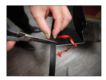
**STEP 9:** Trim any unnecessary extrusion and discard.
