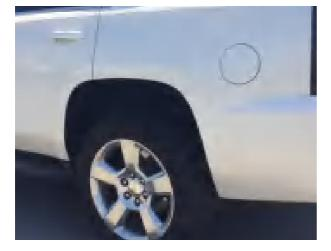
**STEP 10:** Clean the body areas where the Fender Flares will make contact. Ensure all areas are clean and dry before attempting installation.
