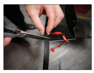
STEP 2: Trim any unnecessary extrusion and discard.
