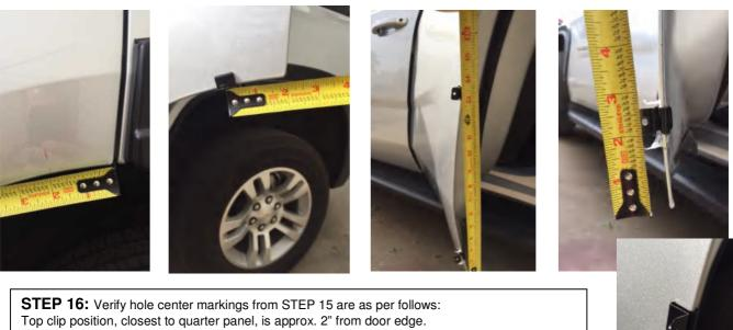
Top clip position, closest to quarter panel, is approx. 2" from door edge. Middle clip position is approx. 13.25" from bottom edge of door. Bottom clip position is approx. 2.25" from bottom edge of door. Apply Mylar tape to marked areas above, half on top surface and half on back surface. Install Slide-on Retention Clips at each location, with the inserted nut facing out and away from the door.
