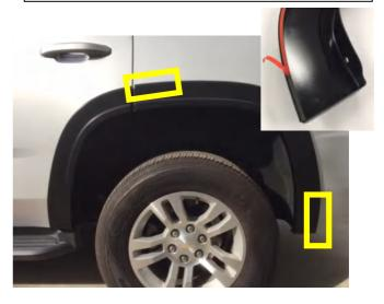
**STEP 13:** Peel back approx. 2" of the adhesive backing from double sided tape that will adhere to the surface of the vehicle, in these (2) noted areas.
