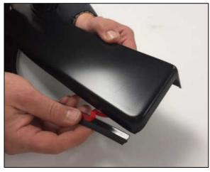
**STEP 1:** Attach the included SINGLE TAPED rubber seal to the Fender Flares. Peel back 2" of the adhesive backing and attach the double sided tape to the inside of the Fender Flare, peeling back a few inches at a time. Ensure pressure is used to secure rubber seal to Fender Flare edge. Attach rubber seal along all areas the Fender Flare will make contact with the vehicle body.
