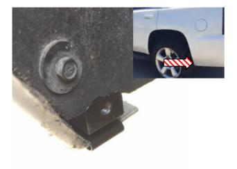
**STEP 12:** Ensure noted area of inner plastic rear bumper is clean. Apply Mylar tape to noted surface ensuring that half goes on top and half on underside where Slide-on retention clip will make contact. Install Slide-on retention clip as shown above making sure it is as close as possible to intersecting corner.
