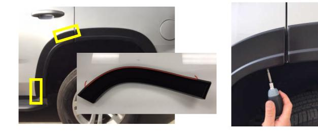
**STEP 17:** Peel back approx. 2" of the adhesive backing from double sided tape that will adhere to the surface of the vehicle, in these (2) noted areas.
