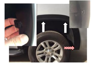
**STEP 14:** Re-install rear quarter panel in position of best fit. Install the (2) "U" retention clips in the uppermost available slots in the Flare ensuring that the barb in the clip engages into the slot of the flare. Use the remaining Machine threaded screw and fiber washer to attach the Flare to the Slide-on retention clip from STEP 12. Pull the exposed tape liners from STEP 13 towards each other and then apply pressure to Flare to adhere double sided tape surface to vehicle fender.
