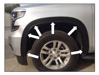
**STEP 4:** Hold Fender Flare against vehicle in position of best fit. Note (6) slots in Fender Flare that correspond with existing screws in vehicle wheel arch and inner splash guard areas. Remove all noted screws with #15 torx driver and retain for later re-installation.
