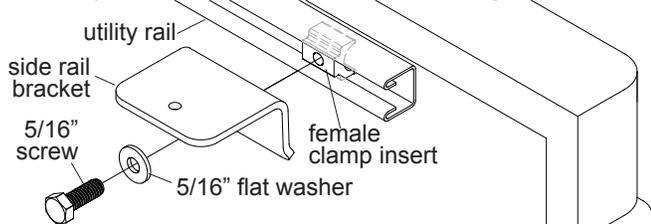
**STEP 3:** Set side rails on side rail brackets. Adjust brackets to align with holes in side rails.
