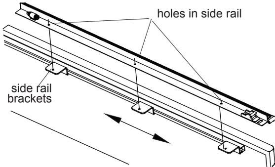
**STEP 4:** Fasten side rail to brackets with 1/4" cap screws, flat washers, and nylon lock nuts.
