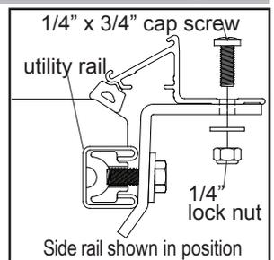
**STEP 5:** Repeat on opposite side. Tighten screws and nuts.
