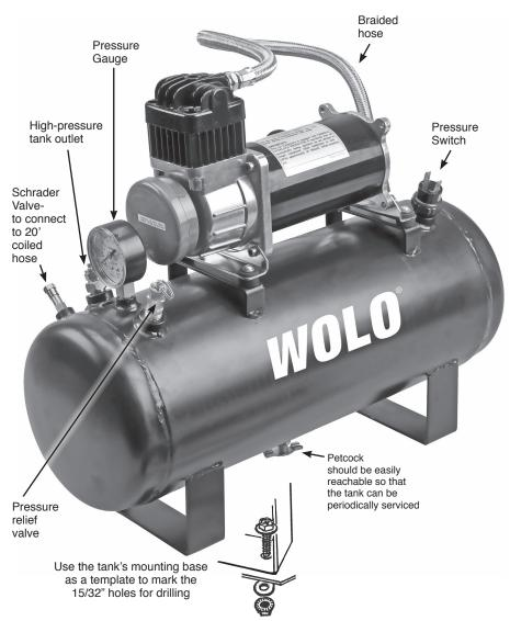
Shown above: Compressor mounted on the tank
