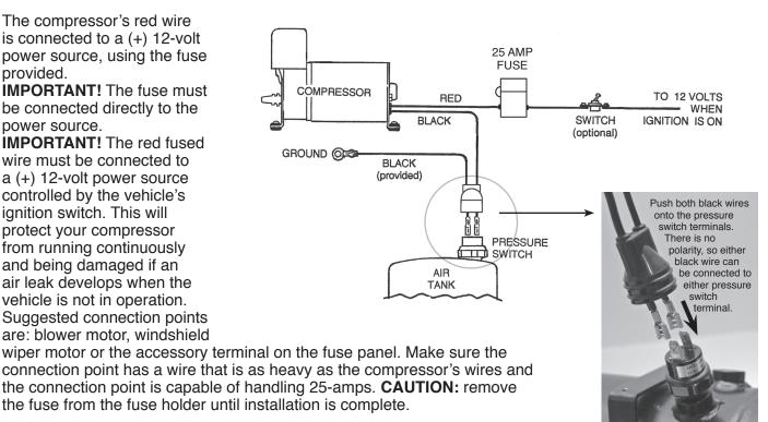
**OPTIONAL:** A switch can be installed into the compressor's red wire. This will permit the driver to turn-off the system if it is not required. (Fig. 7)
