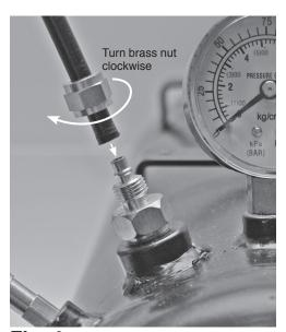
Fig. 4 Connecting the high-pressure plastic hose
