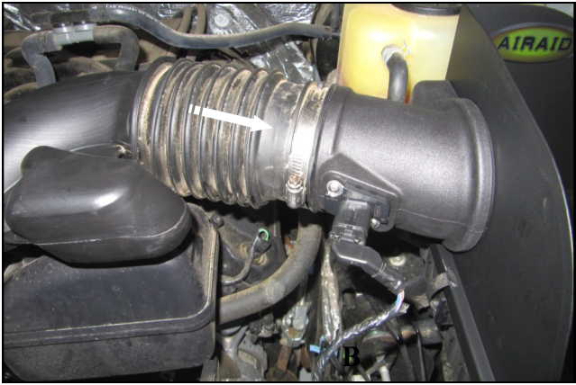
12. Slide the factory intake tube onto the Airaid Tube and tighten the clamp. Reconnect the Mass Air Flow or MAP sensor.
