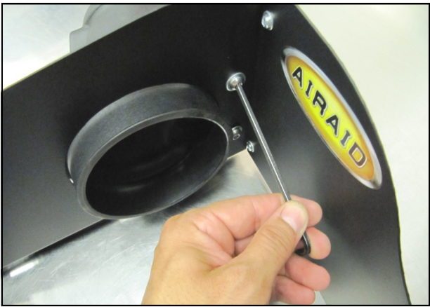
10. Install the Air Meter Tube into the Panel Assembly and secure using the two 1/4-20 Button Head Screws ,and 1/4” Flat Washers .
