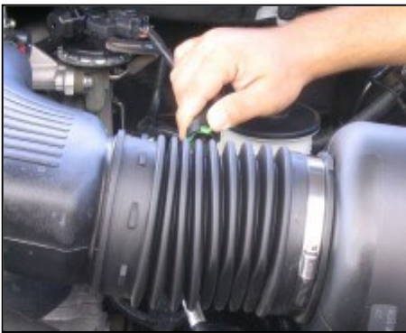
14. Disconnect valve cover breather hose from factory intake tube and valve cover.
