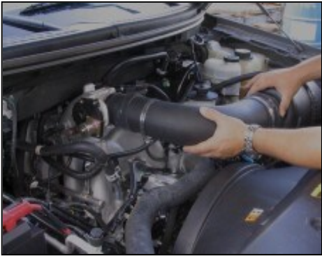
19. Install the Airaid Modular Intake Tube on engine.
