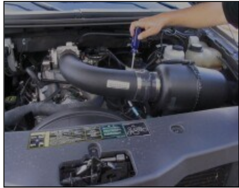
20. Tighten hose clamps on both ends of the Modular Intake Tube.
