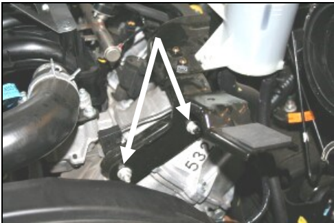
17. Factory tolerances may require adjusting the factory bracket to align the tube and hump hose with the filter adapter. Therefore, it may be necessary to loosen the two mounting nuts with a 13mm deep socket, and adjust it.
