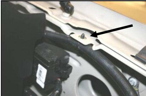
18. Slip the black plastic hose mount (#26) over the radiator overflow hose. Next, place one 1/4" flat washer (#15) over the hole on the inner drivers side fender. Slide the hose mount prongs thru the fender and thru the washer.
