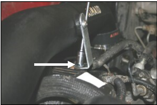
20. Install the 6mm bolt (#15), and 1/4" flat washer (#12), thru the L-bracket, and into the valve cover, adjust for fit, and then tighten all hose clamps, and bolts.
