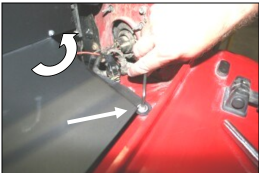
15. Install the supplied 1/4" button head bolt (#11), and 1/4" washer (#12), thru the CAD, with the 1/4" fender washer (#13) and nut (#14), on the bottom of the fender. Re-install the factory bolt in the radiator shroud removed in step #9.
