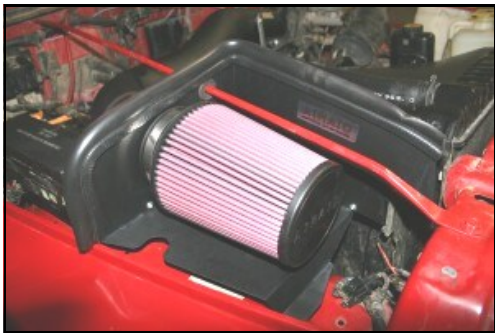
22. Install the Airaid Premium Filter (#1) onto the CAD tube and tighten the hose clamp. Next, install the weather strip onto the top of the CAD as shown, starting at the fender, working your way towards the radiator.
