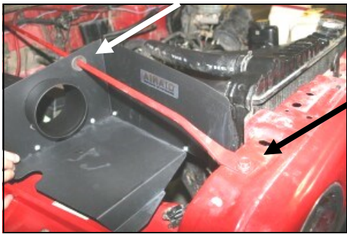
13. Align the CAD over the mounting holes, and re-install the factory bolt from step #10 in the radiator support. Slide the grommet forward into the hole in the CAD as shown.
