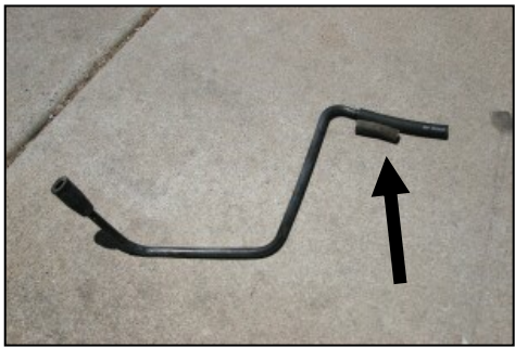
13. Remove the factory hose from step 2, and install the new 3/8"x 4" hose on the end of the vacuum line as shown. Reinstall vacuum line. (Refer to step 2.)
