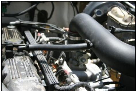
17. Replace the factory breather hose with 1/2"x10" rubber hose between valve cover and intake tube using speed clamps as shown.
