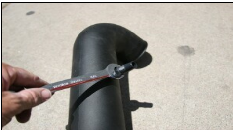
14. Install the 1/4" barbed fitting into the intake tube.
