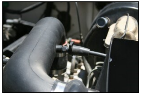
16. Slide intake tube into the hump hose first, and then into the coupler. Adjust for a good fit, and tighten hose clamps. Slide vacuum hose on barbed fitting, and install speed clamp as shown.
