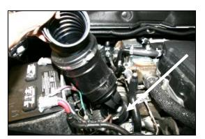
**5.** Loosen the factory hose clamp at the base of the factory plastic intake tube assembly, and remove the tube from the vehicle.
