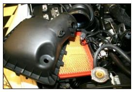
**2.** Unsnap the two metal clips that hold the airbox lid to the base, and remove the lid. Next, remove the factory paper air filter from the base.
