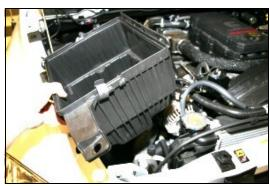
**4.** Gently rock the airbox base back and forth while pulling up, to remove it from it's mounting grommets, and remove it from the vehicle.
