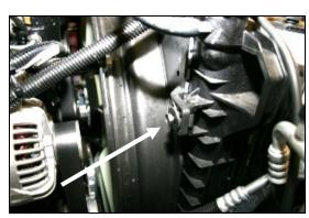
**6.** Using a 13mm socket, remove the factory bolt that holds the fan shroud to the radiator.
