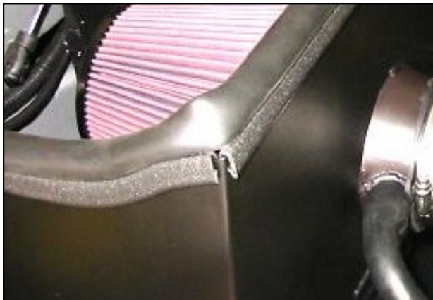
18. 2004-05 Models Only: Connect the factory breather hose to the Airaid Cool Air Dam & secure using the #24 Speed clamp provided.
