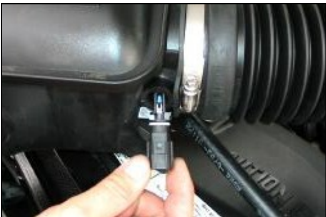
6. 2003-05 Models Only: Disconnect air temperature sensor wire on back of factory throttle body air chamber and remove sensor. Retain sensor for later use with the Airaid Intake System.
