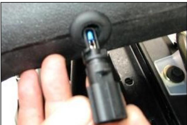
9. 2003-2005 Models Only: Install rubber grommet w/thru hole and insert the factory air temperature sensor into the grommet.
