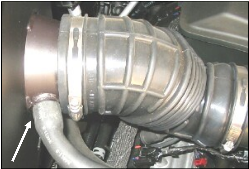
6. 2004-2005 Models Only: Reconnect the factory breather hose to the nipple on the CAD and secure it using one #24 speed clamp (#4).
