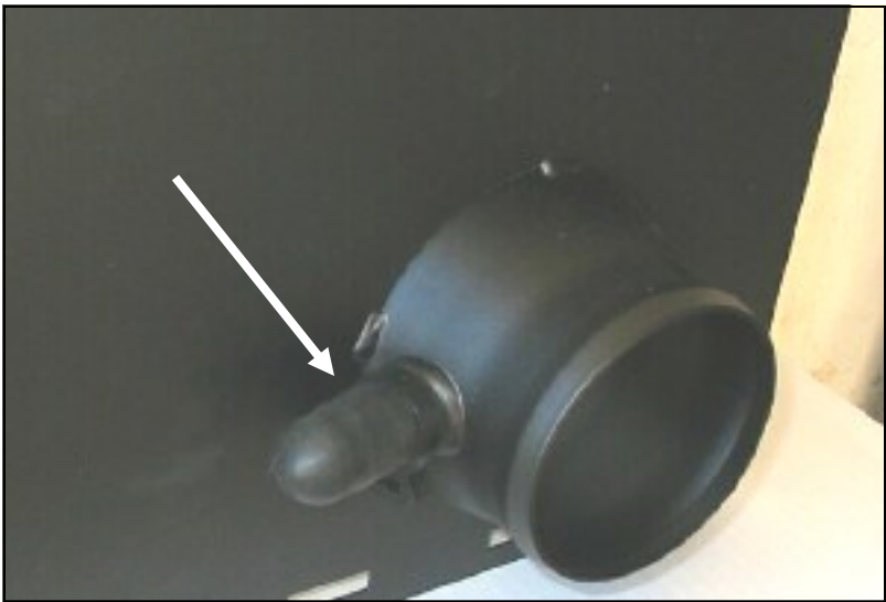
5. 2002-2003 Models Only: Slip the black rubber cap (#6) over the nipple on the CAD and secure it using one #19 speed clamp (#5).
