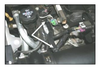
12. Slide one end of the 3/8" x 8" breather hose (#16) over the barbed fitting in the Airaid Intake tube. Slide the other end of the breather hose onto the metal tube on the engine.
