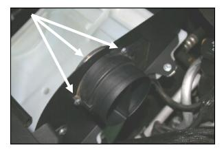
**8.** Mount the **MAF** sensor onto the panel using three  $8-32 \times 1/2$ " button head screws (#11), #8 flat washers (#12), and 8-32 keps nuts (#13). (Note: sensor should be mounted with "flow" arrow on top).
