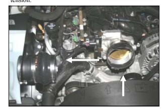
9. Slide the silicone hump hose (#4), and two #56 hose clamps (#14) onto the MAF sensor. Slide the coupler (#5) and one #68 hose clamp onto the throttle body. Tighten only the clamp on the MAF sensor for
