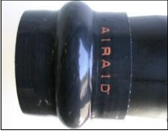
12. Install the provided urethane hump hose (#7) onto the Airaid Modular Intake Tube (MIT) (#5) with the 2 supplied #60 hose clamps (#11). Note: Leave hose clamps loose until final assembly.
