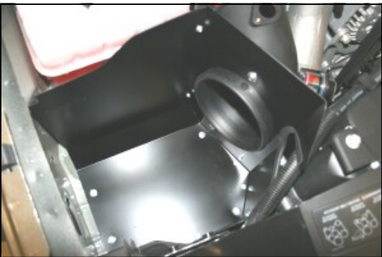
11. Install the assembled CAD into the vehicle where you removed the factory mounting plate in step #6. Use four bolts (#9), and washers (#7) to secure the CAD. Do not over tighten the bolts.
