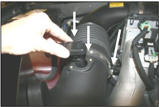
12. Re-position the factory intake tube onto the Airaid tube, and tighten the hose clamp. Next re-install the Mass Air Flow sensor into the Airaid tube using the two provided Button Head screws (#8). Do not use the factory screws! Do not over tighten!
