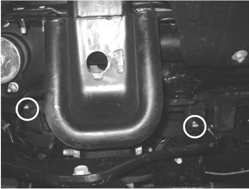
4. Remove bottom 4 grille screw from underneath truck with 10mm wrench. The 2 driver side locations are shown above. Repeat on passenger side.
