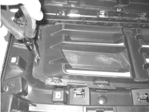
10. Use needle nose pliers to squeeze clip and snap out top and bottom factory grille inserts.
