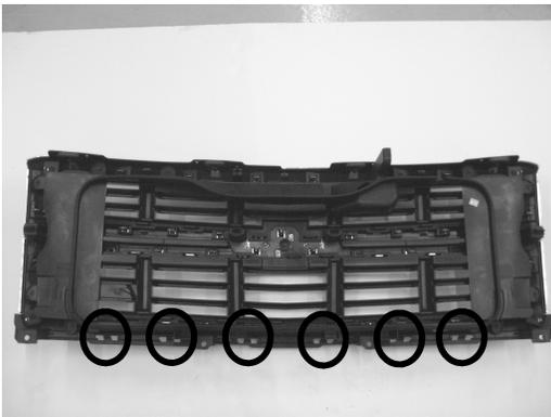
8. Once grille and upper bumper are off the truck. Remove the upper bumper piece from grille. Use a flat head screw driver to unclip the 6 tabs on bottom backside of the grille.
