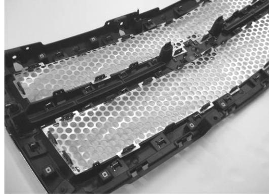
11. Snap in top and bottom Putco grille insert into grille over existing tabs.
