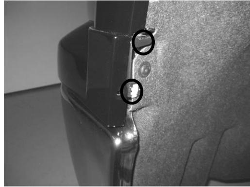
5. Remove 2 bolts in front wheel well on the upper bumper. The driver side locations are shown above. Repeat on passenger side.
