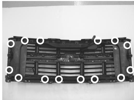
9. Remove shroud from behind grille. Use 7mm wrench to remove 14 bolts.
