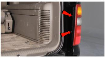
2) Remove [2x] Phillips Bolts securing the tail light.
