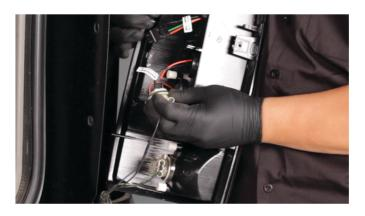
8) Connect the turn signal socket to the center socket insert of the Spyder tail light. Align the black wire side of the socket with the black wire side of the insert to ensure correct polarity. Reinstall the socket.
