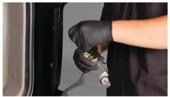
6) Remove the brake lamp bulb from its socket. Never touch exposed bulbs with bare hands.
