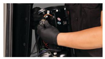
9) Connect the brake lamp socket to the upper socket insert of the Spyder tail light. Align the black wire side of the socket with the black wire side of the insert to ensure correct polarity. Reinstall the socket. Your Spyder LED tail light is now ready to install.
