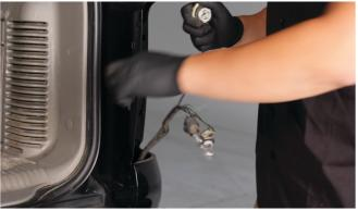
5) Remove the turn signal bulb from its socket. Never touch exposed bulbs with bare hands.
