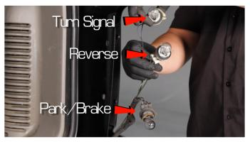
4) Remove the turn signal, reverse lamp and brake lamp bulb sockets from the OEM tail light. Never touch exposed bulbs with bare hands.
