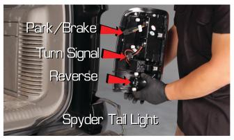
7) Install the reverse lamp socket into the Spyder tail light.
