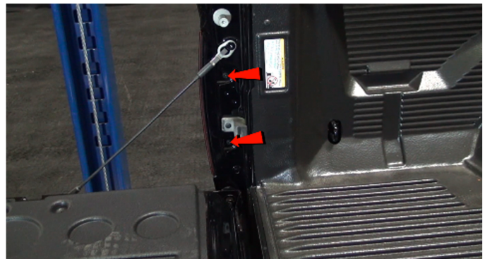
2) Remove [2x] T-15 torx screws securing the tail light.
