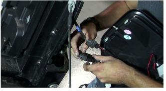
4) Locate your SPYDER tail light. Connect the OEM wiring harness to your SPYDER tail light. Be sure to install the reverse lamp bulb socket.
