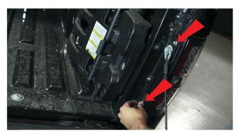
6) Reinstall the two 8mm bolts to secure the tail light.
