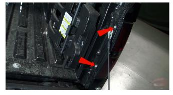
1) Open the tailgate. Remove the two 8mm bolts securing the tail light.
