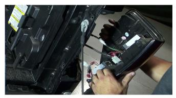
3) Disconnect the brake light and turn signal wiring harnesses, then remove the reverse lamp bulb socket.
