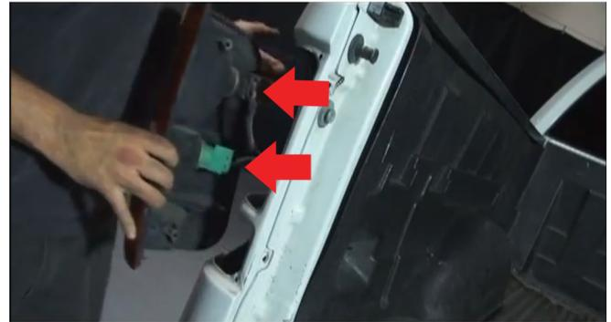
2) Next, gently pull outwards from the side of the tail light to remove freely. Still attached will be the tail light harness (arrow). Remove both bulb sockets by twisting counter-clockwise. Retain the reverse light bulb and only remove the turn signal bulb from the socket.
