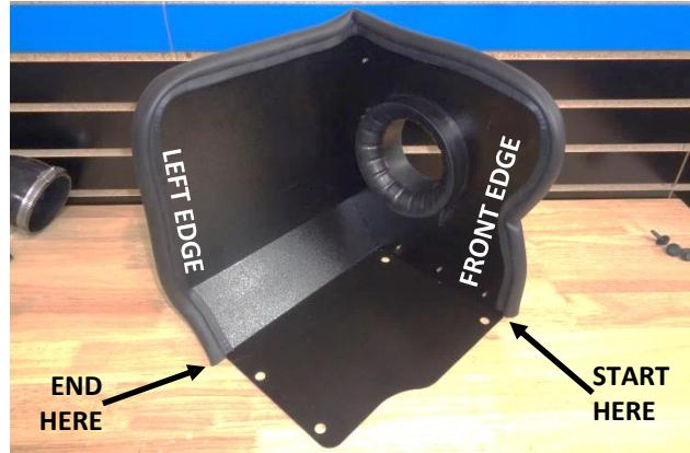
16. Attach the gasket (5) to the heat shield. Starting at the bottom of the front edge, firmly press the seal onto the edge, gradually working your way around. At the bottom of the left edge, use metal-cutting shears to trim the seal to fit.
