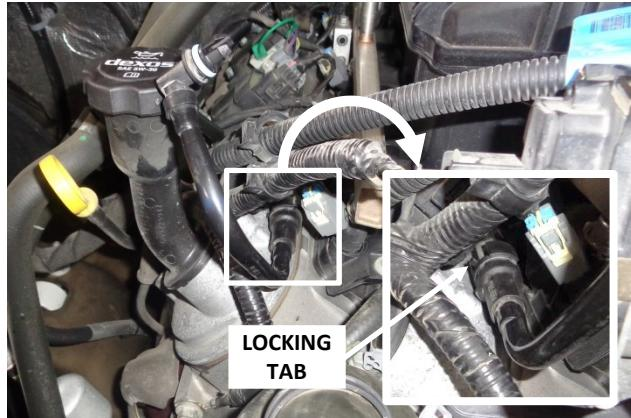
10. Remove the PCV tube from the engine end by releasing the locking tab and pulling the line straight off.
