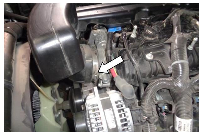
5. Loosen the screw clamp securing the intake duct to the throttle body.
