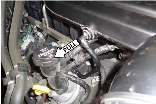
7. Disconnect the PCV tube from the left side of the air duct by pulling it straight outward.
