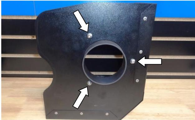
15. Assemble the air filter adapter (3) to the heat shield (4) using the M6 screws (8), lock washers (7) and flat washers (6).
