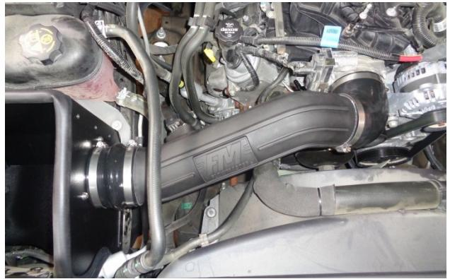
22. Install the intake tube in the vehicle.
