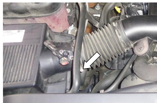
6. Loosen the screw clamp securing the airbox to the intake duct.
