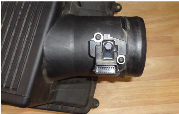
13. Remove the MAF sensor from the airbox, then remove the sensor gasket. **CAUTION: The sensor is delicate!** Handle it with care, and keep it in a safe location until reinstallation.
