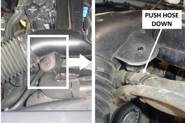
8. Separate the hose clamp from the intake duct by carefully pushing down on the large coolant hose.
