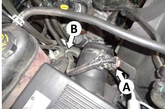
11. Disconnect the electrical plug from the Mass Airflow (MAF) sensor (A) by pulling the locking tab away from the sensor and pulling the plug straight off. Disconnect the MAF sensor lead clip (B) from the airbox.
