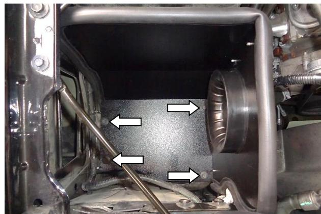
17. Use the 4 bolts removed at Step 14 to install the assembled heat shield in the vehicle. **NOTE: If the bolts are different lengths, be sure to use the correct length bolt at each location, as determined at Step 14.**
