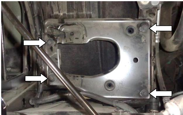
14. Remove the airbox shelf by removing its 4 mount bolts. Retain the bolts for reinstallation at Step 17. **NOTE: If the bolts are different lengths, note the length of each bolt and its location, to maintain proper bolt clearances at reinstallation.**
