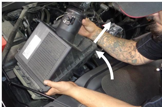
12. Remove the airbox by lifting up its inboard side (to release the mount pins from their rubber grommets), then sliding the airbox inboard (to release it from its shelf).
