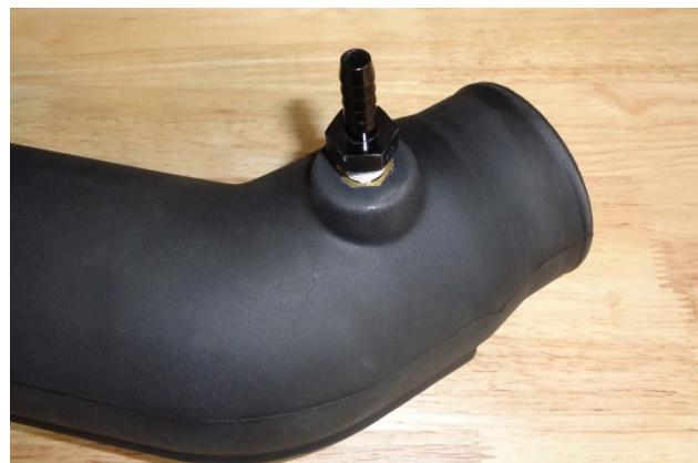
18. Apply 2 wraps of nylon thread tape to threads of the 3/8" barbed fitting (13), and install it in the intake tube (14).
