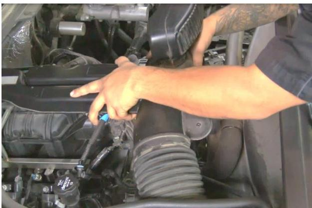
9. Separate the intake duct from the airbox and throttle body, and remove the duct from the vehicle.
