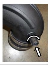
14.Install the provided rubber grommet into the hole on the FM intake tube and insert the previously retained air temperature senor fully by twisting clockwise and pressing in at the same time.
