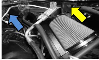
16. Reinstall the two previously removed bolts on the fender → and the front cross-frame → to secure the FM air-intake assembly. Check all fitment /fasteners and reattach the negative battery cable. Enjoy!
