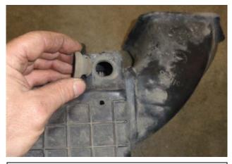
5. Turn the stock air intake assembly over and remove one of the rubber grommets from the base and retain for use on the FM Cold Air Intake System.
