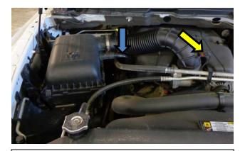
2. Disconnect the air-temperature sensor plug on the intake tube by depressing the rocking tab and gently pulling away. Next, disconnect the crankcase breather hose from the stock air-box. NOTE: We highly recommend that customers retain their factory air intake system.
