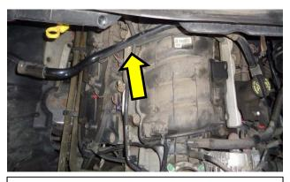
7. Remove the crankcase vent tube from the engine. Replace the stock tube with the included hose/clamps. Route in the same path, trimming off any excess length after install of the FM system.
