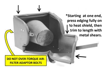
12. Using the (3) three 6mm bolts/washers, secure the air-filter adaptor to the heat-shield assembly. Next, install the rubber edging as above \*, then securely attach the provided FM air-filter/clamp assembly. If desired, install pre-filter over the cone element. This will help extend the life of the filter by keeping out the larger particles.
