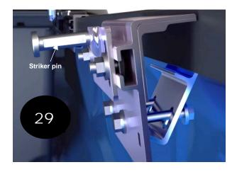
The rear bed rails are unique to the left and right side of the truck. Ensure that the striker pin is positioned towards the rear.
