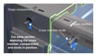
Lift the rear of the compartment upward to allow the cross member to be slid into the channel on the underside of the flange.
