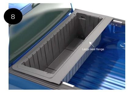
Place the cargo compartment into the front of the truck box. The large seal flange is positioned towards the rear of the truck.
