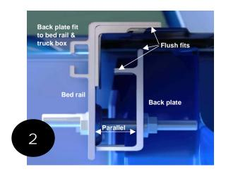
Raise the bed rail back plates <u>until flush</u> with the underside of the truck box while keeping it parallel to the back side of the bed rail.
