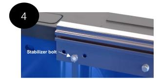
Loosen the jam nut and thread the stabilizer bolt through the bedrail until it firmly contacts the truck sheet metal behind the bedrail.
