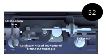
Loosen the two striker nuts holding the striker in the shipping position on the rear bed rails.
